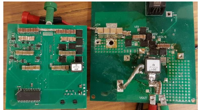
Fig. 14. Size Comparison for Two-Phase ZIV Converter Prototype versus early 7-Switch prototype in [8]
